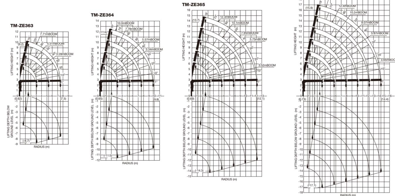
Note: The above lifting heights and boom angles are based on a straight (unladen) boom, and allowance should be made for boom deflection obtained under laden conditions.
